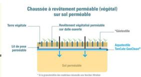
Exemple de chaussée perméable (Source: [tencategeoclean.com](http://tencategeoclean.com))
